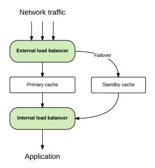
In addition to the cache failover shown in the diagram to the left HeartyHosting also includes automatic failover instances for backend databases, such as MySQL, web servers and file systems.
